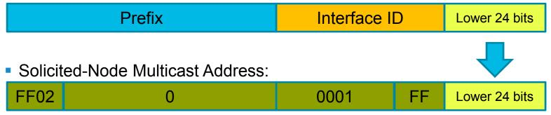
Solicited-node address is a link local multicast that has the target node's least significant 24 bits within it
