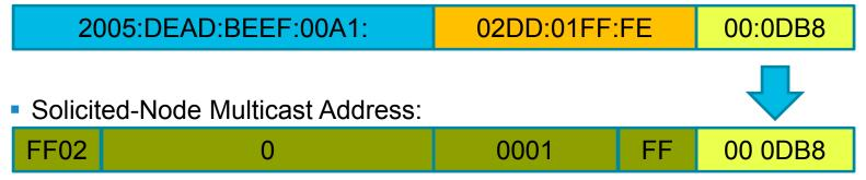
The conversion of layer 3 multicast to layer 2 is to take the last 32 bits of the IPv6 address and prepend 33 33
